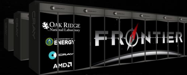
2022: Cray Frontier: >1 Eflops, AMD GPUs, Burst Buffer Storage 10TB/s, long term at 4.6 TB/s, 21MW
