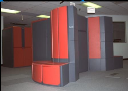
1988: Cray Y-MP: 2.7 Gflops: Vector Processors, SSD storage (13.6 GB/s)
