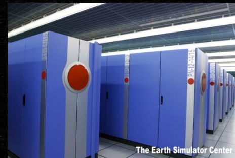
2002: Earth Simulator 40 Tflops, 50MW, vector procs
