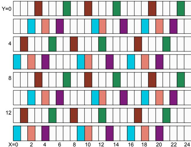
**Fig. 2. Topological XY representation of Titan’s Lustre routers.**
